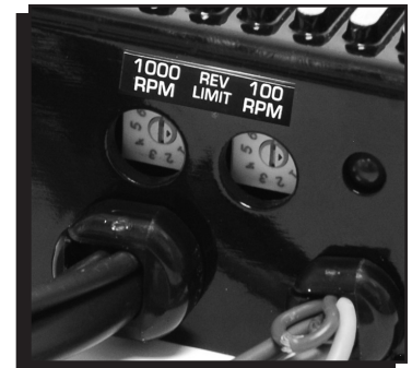
Figure 3 Adjusting the Rev Limiter.
